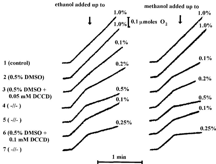
Fig. 2. The effect of solvents and DCCD on  $O_2$  evolution in the presence of MV. Left traces: effect of ethanol; right traces: effect of methanol. Curves 1: control (reaction mixture as in Fig. 1); curves 2: reaction mixture contains 0.5% DMSO; curves 3, 4, 5: reaction mixture contains 0.5% DMSO + 0.05 mM DCCD; curves 6, 7: reaction mixture contains 0.5% DMSO + 0.1 mM DCCD.
